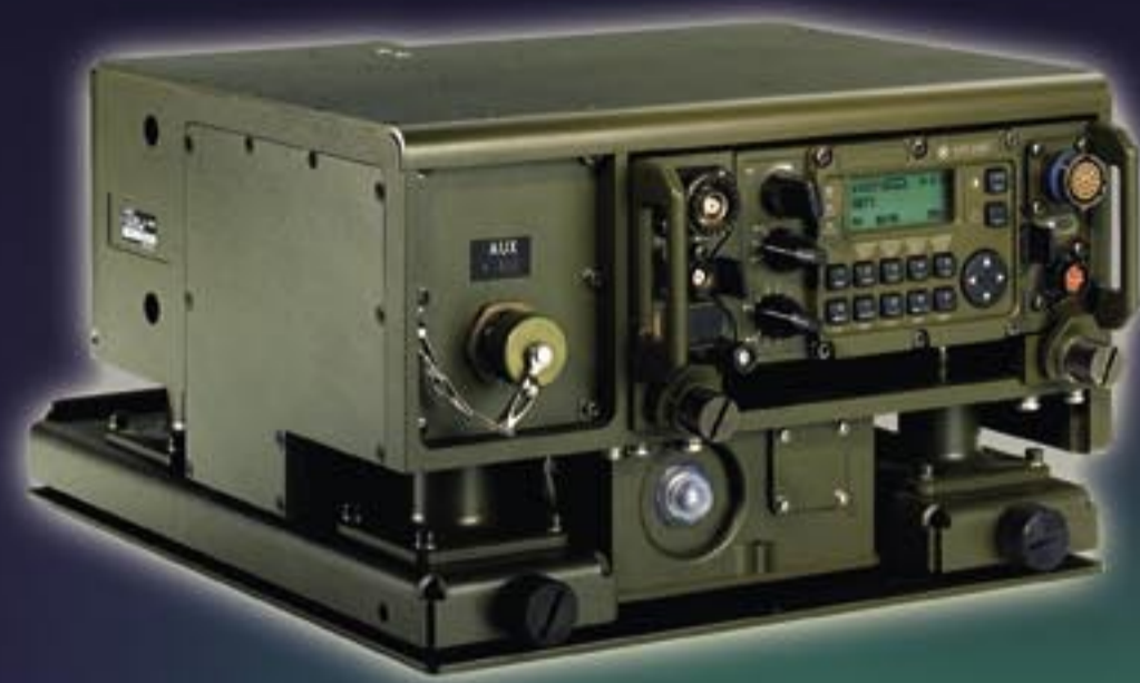
R&S®KG3031A Single Docking Station for R&S®M3TR Manpack Radios
